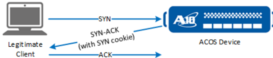
Figure 1 : SYN-ACK Handshake (Legitimate Client)
