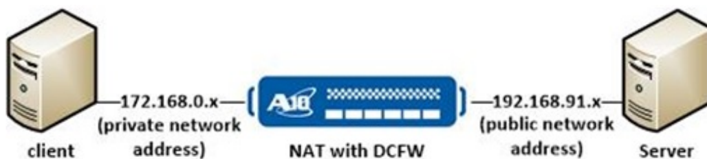
Figure 4 : Network topology diagram for NAT with firewall
