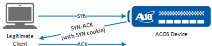
Figure 25 : SYN-ACK Handshake (Legitimate Client)
